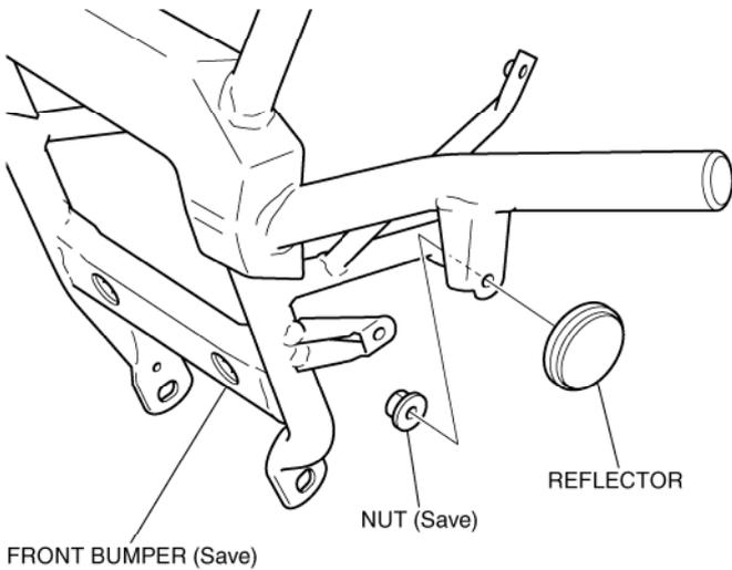
5. Install the reflector as shown.
