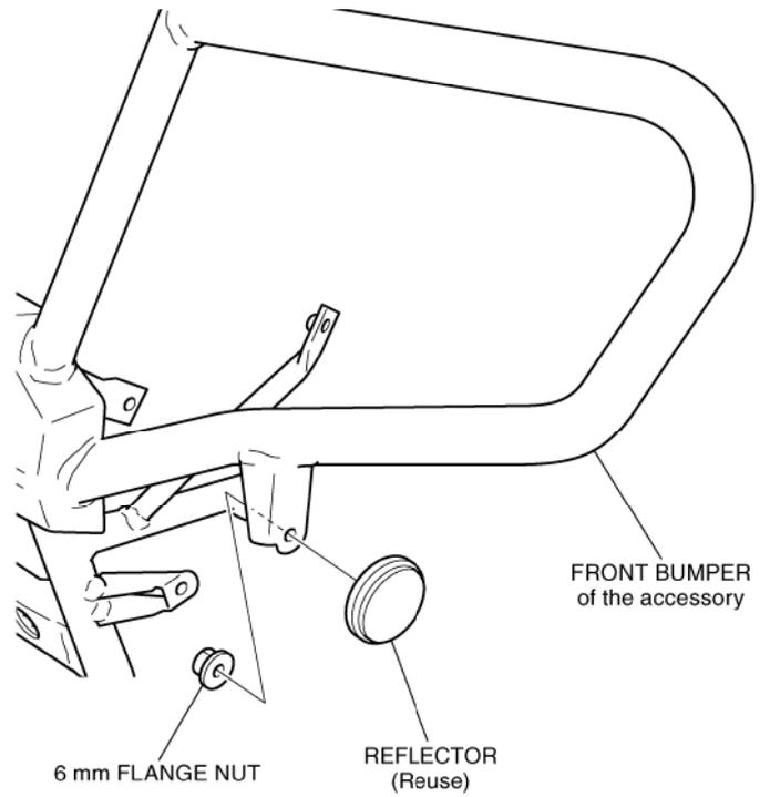
6. Install the front bumper of the accessory in the reverse order of removal.
