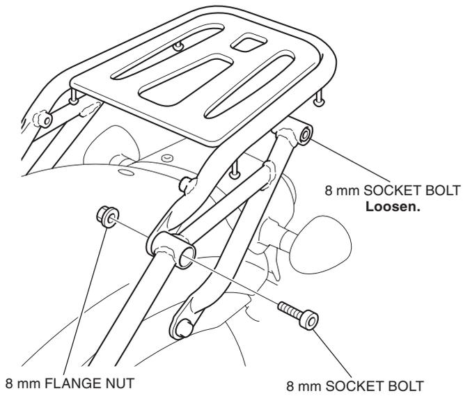
4. Install the backrest assembly as shown.
