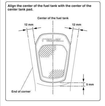
Apply adequate pressure to the attached center tank pad.
