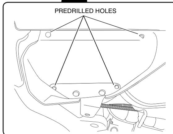
3. The net crimps should toggle once they go through the holes, and they should not be able to come back out of the holes so that the side pocket net remains in place.
