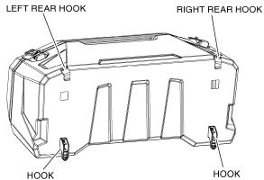
Lift the lever on each Pro-Connect<sup>™</sup> latch to unlock them and slide the Rubber Spacer around the Pro-Connect<sup>™</sup> latch. Insert the Pro-Connect<sup>™</sup> latch, spacer and snap ring assembly in the cargo box square hole.
