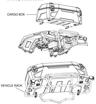
4. Secure the cargo box to the vehicle by pressing down each Honda Pro-Connect™ latch lever.
