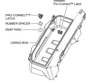
3. Lift the lever on each latch to unlock them. Place the cargo box onto the rear rack of the ATV. Line up each latch with its corresponding hole in the rack then push each latch into its hole. Before and after cargo box installation on the vehicle rack are shown on the pictures below.
