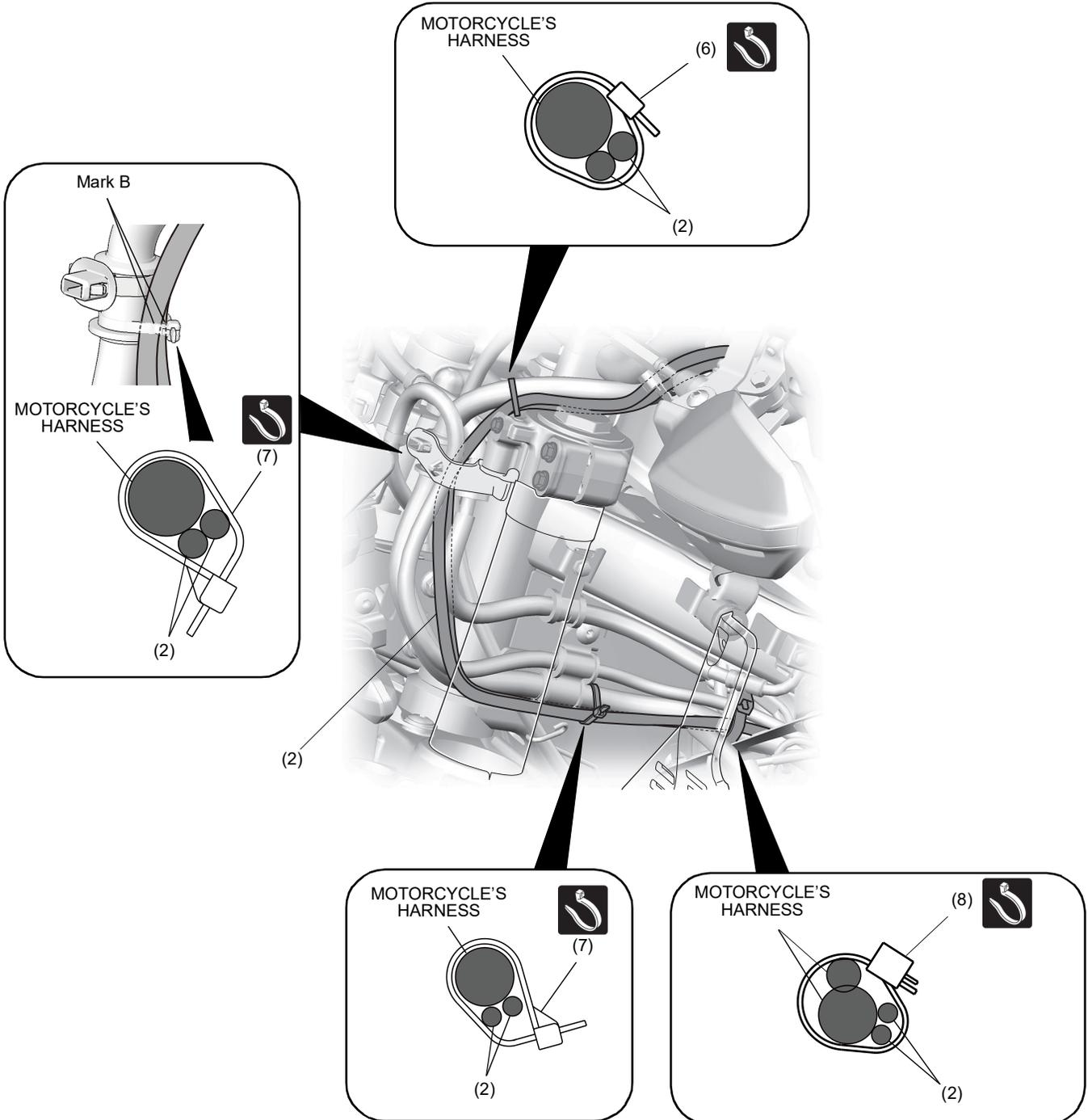
7. Apply grease and install the parts as shown.
