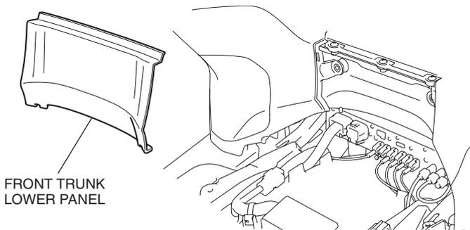
10. Remove the parts as shown.
