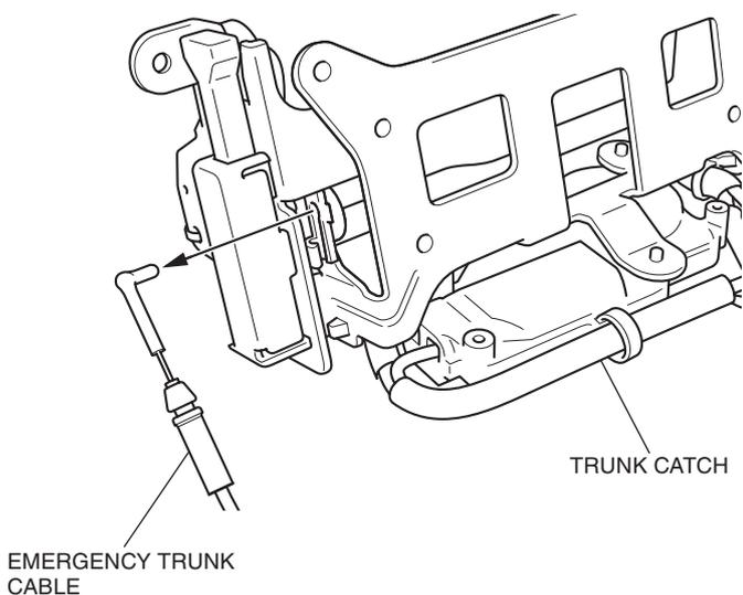
21. Remove the trunk sub assembly as shown.
