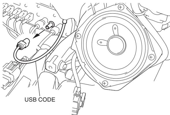
16. Disconnect the connector as shown.
