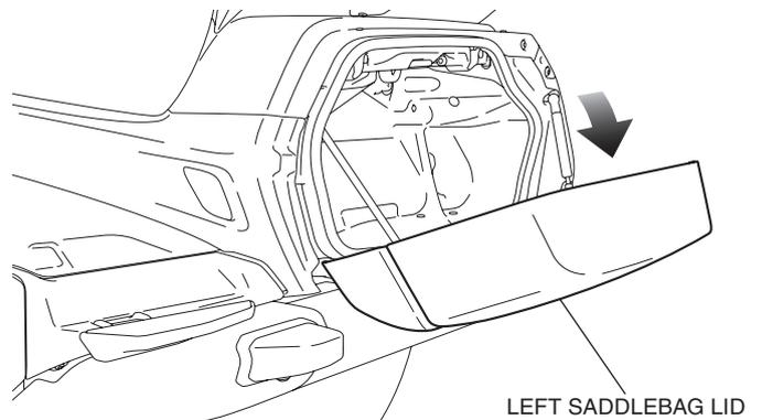
2. Remove the left side cover as shown, and disconnect the negative (-) cable of the battery.
