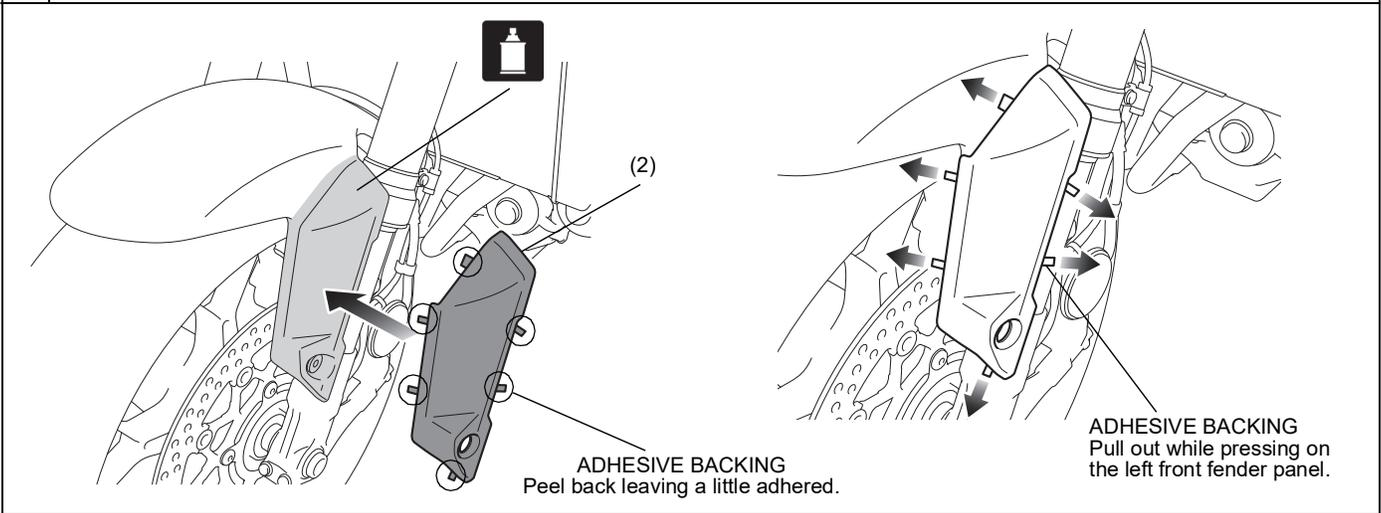
3. Install the parts as shown.
