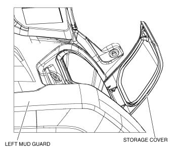
2. Using a flat-head screwdriver, separate the storage cover from the storage compartment at the attachment points.
