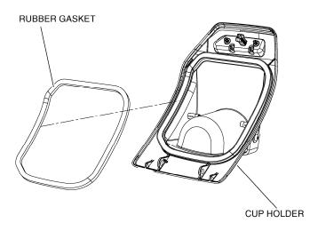
4. Attach the cup holder to the storage compartment using the attachment points shown in Step 2.
