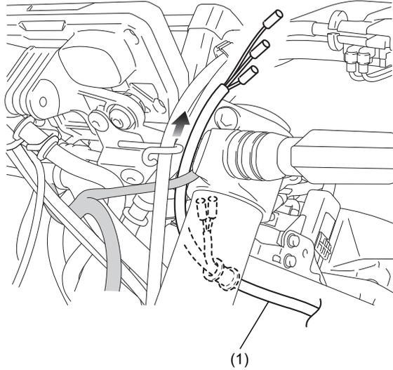
10. Connect the harness and secure with electrical tape as shown.
