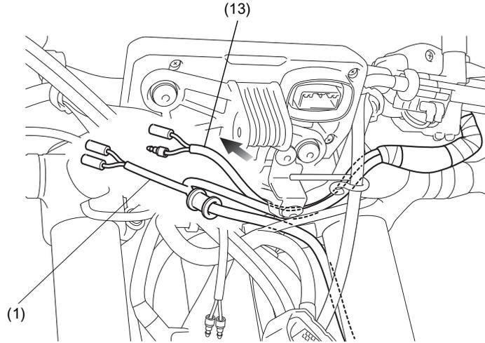
12. Wrap the terminals with electrical tape as shown.
